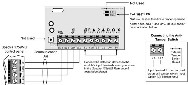
Remove AC and battery power from the control panel before connecting the module to the communication bus. Do not connect the APR3-ZX4 or SPC-ZX4 more than 76m (250ft) from the control panel. Only one APR3-ZX4 or one SPC-ZX4 can be connected per Spectra control panel.
