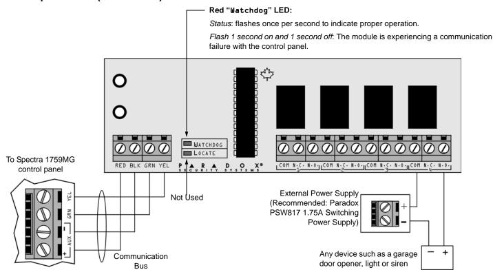
Remove AC and battery from the control panel before adding the 4-PGM Output Module to the system. Do not connect the APR3-PGM4 more than 76m (250ft) from the control panel. Only one APR3-PGM4 can be connected per Spectra control panel.
