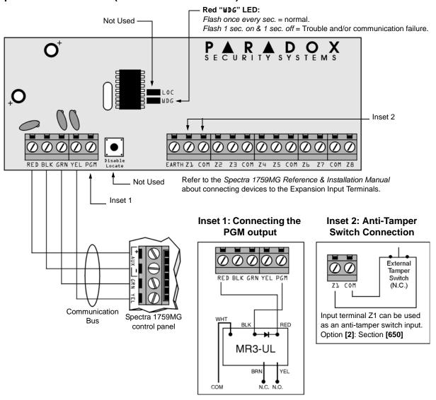
Remove AC power and battery before adding a module to the system. Do not connect the APR3-ZX8 or SPC-ZX8 more than 76m (250ft) from the control panel. Only one SPC-ZX8 or APR3-ZX8 can be connected per Spectra control panel.
