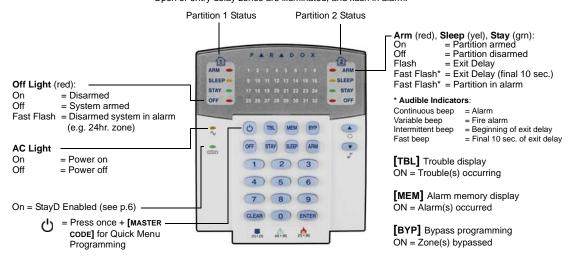
Figure 3: MG32LRF (32-zone Wireless LED Keypad Module)
