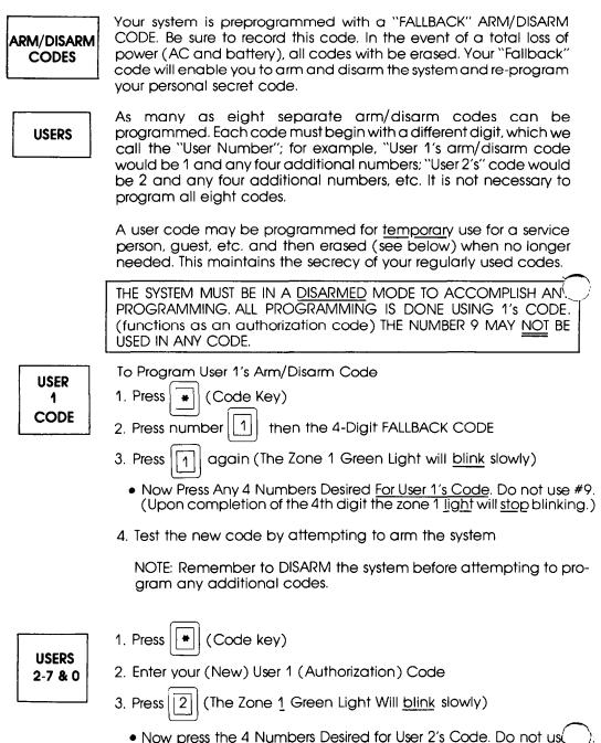
(Upon completion of the 4th digit the Zone 1 light will stop blinking.)
