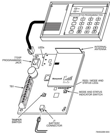
**Figure 10. Cable Connections**
