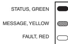
**Figure 11. Unregistered 7845GSM Status Display In Normal Operation**
