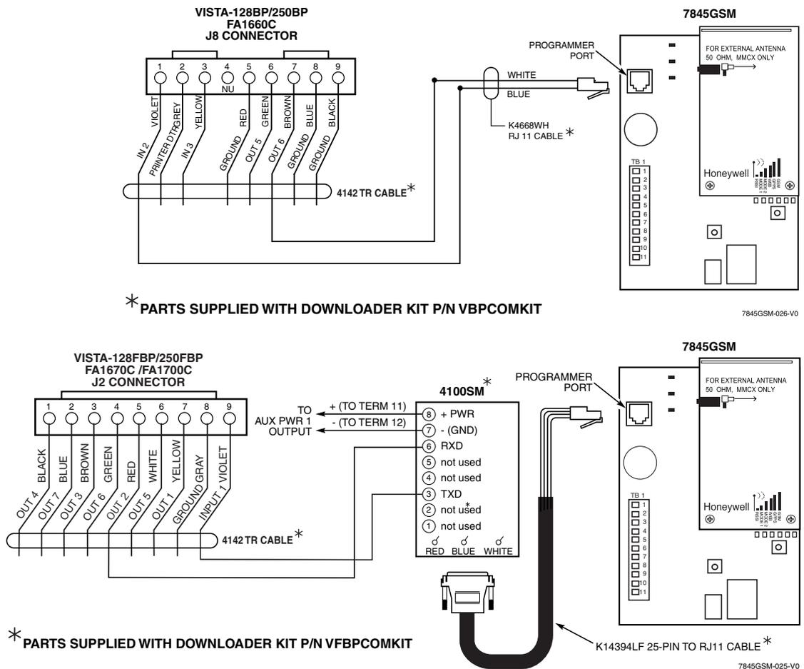
Figure 17. Cable Connections for Direct Wire Downloading
