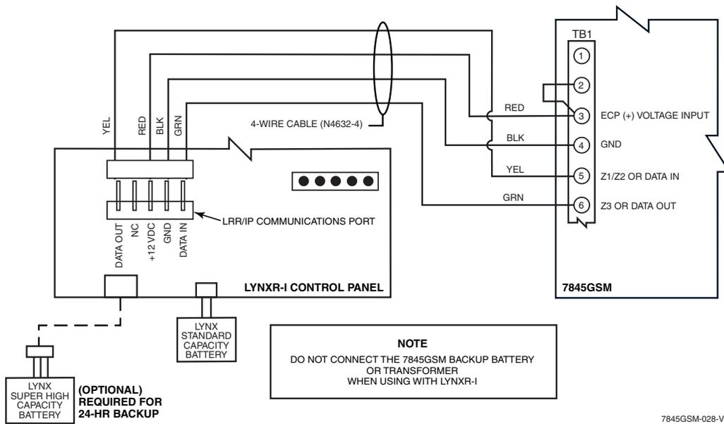
**Figure 3. Wiring a LynxR-I for ECP Mode**
