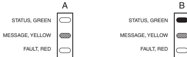
**Figure 15. A Registered 7845GSM Status Display (A) and an Unregistered 7845GSM Status Display in Normal Operating State(B)**
