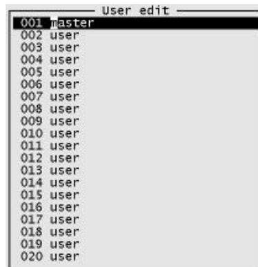
Use the h and g keys to scroll through the list of users. The cursor will be flashing on the default user name. To insert a new users name, simply type in the name. To assign ID codes and options press n. The user options list is displayed.
