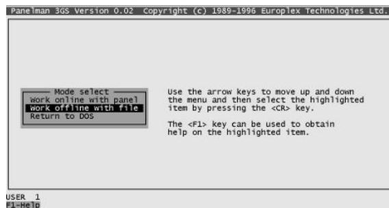
Highlight WORK OFFLINE WITH FILE and press f. To work on an existing file select one from the displayed list and go to page 15. Three of the seven ON LINE menu options are available.
