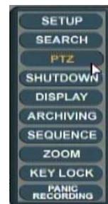
Speed domes and other telemetry devices connected to the DVR, can be fully controlled from the front panel. In live display mode, press the **PTZ** button. To select a camera to control, use the **CHANNEL SELECTION** buttons. Pan and tilt movement is controlled by the **CURSOR KEYS**, zoom is controlled by turning the **SHUTTLE WHEEL**.
