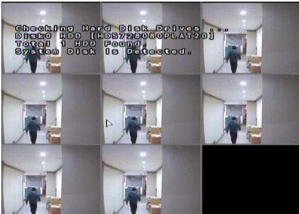
The DVR startup screen detects and checks the status of hard drives and the CDRW / DVR-RW drive.
