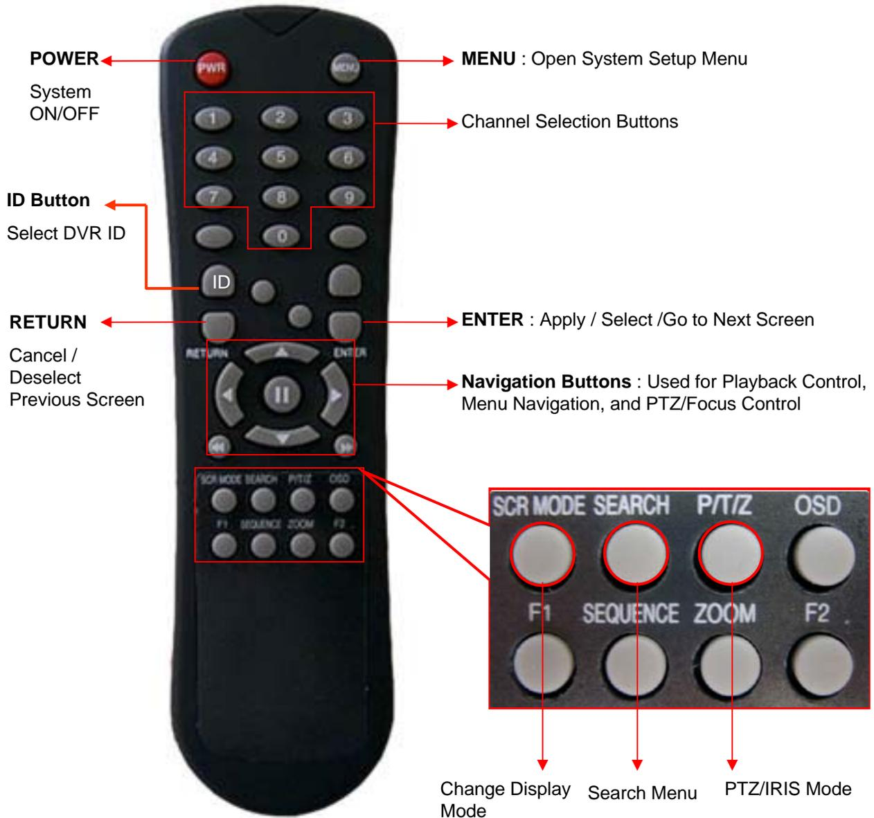
※ If there are many DVRs on stack, each DVR must be set different ID then Remote controller set each ID on DVR. Can control all DVRs on one Remote controller by each ID.
