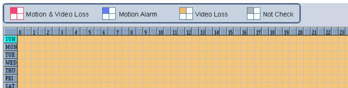
1. Motion & Video Loss (Red): DVR System responds with Motion Detection and Video Loss alarm in specified time.
