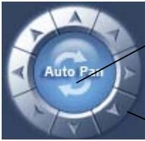
Pressing this button initiates the connected PTZ camera to do an automatic tour of 360, but for speed dome, many PTZ factory forbid this command.
