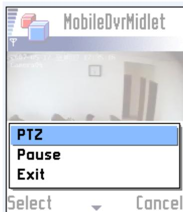
Press the “Options” button and select the “PTZ” button to enter the PTZ control interface.
