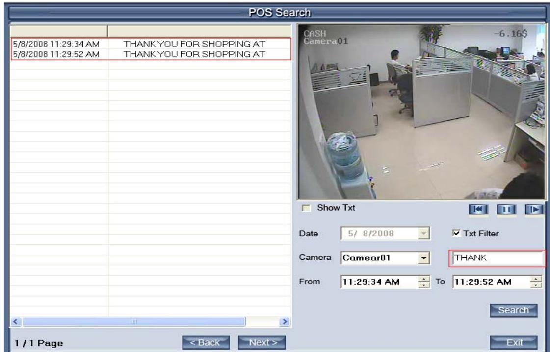
The word of the TXT.Filter is THANK,then,press the Search ,the content display all the Pos messages with the “THANK” From.. To: Select the begin time and the end time
