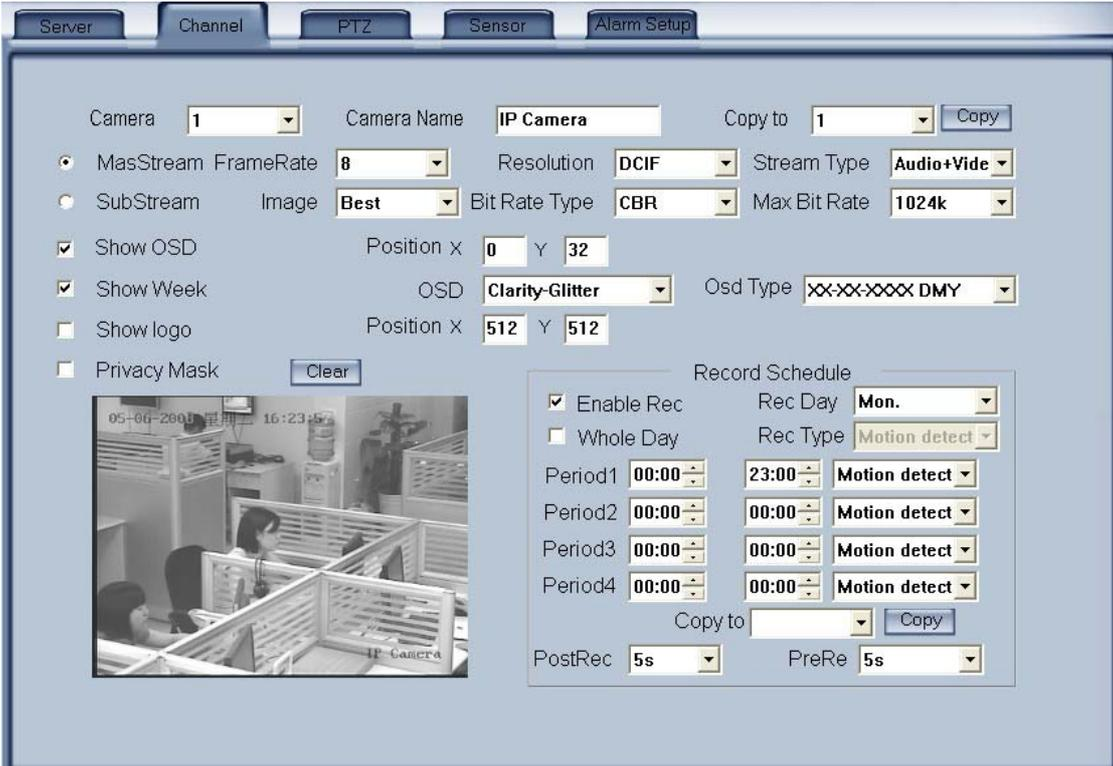
This section contains the parameters to designate a name for every camera connected, to enable or disable show LOGO and OSD, and to set display type of OSD & LOGO as well as record resolution, record type, record quality and frame rate, etc.
