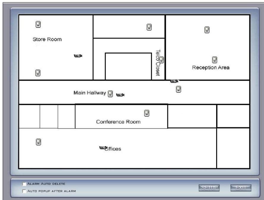
If it is set to appear automatically, when the sensor is triggered, the map will appear automatically and the sensor being triggered will be marked. For triggered camera, user can Left-Double-Click it to view its video.
