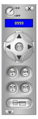
Figure 6-24 PTZ control panel
