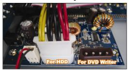
Step 4: Fix the HDD to the bracket with the PCB side facing up, and replace the HDD bracket back to the DVR base.
