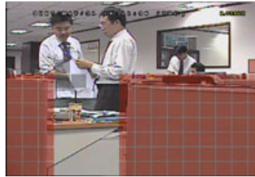
You can also set up multi-detection area.
